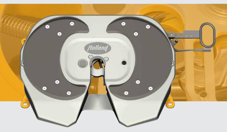
The grease-free HOLLAND NoLube technology offers many new possibilities: The 20t class is especially light and lubricant free and sets new standards.
